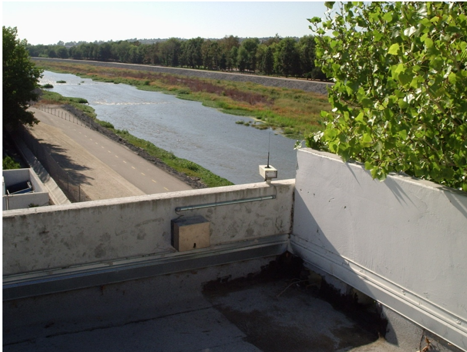
Figure 3 Photo of the Recreational Use Survey Camera Installation for Santa Ana River at Anaheim
