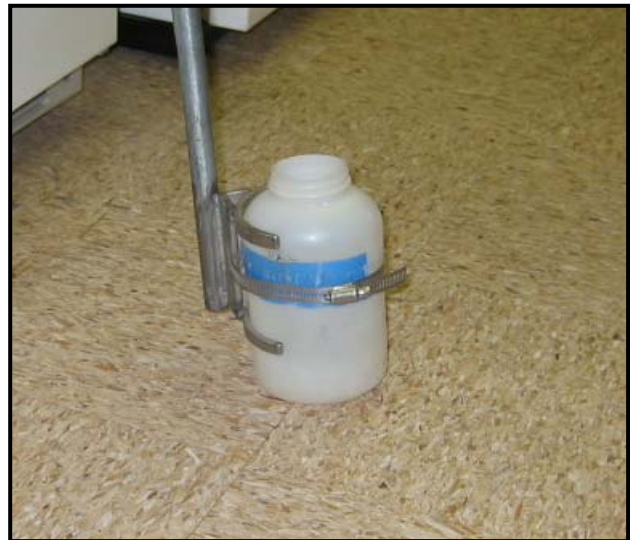
Figure 5-2 Close-up of Samplina Pole
